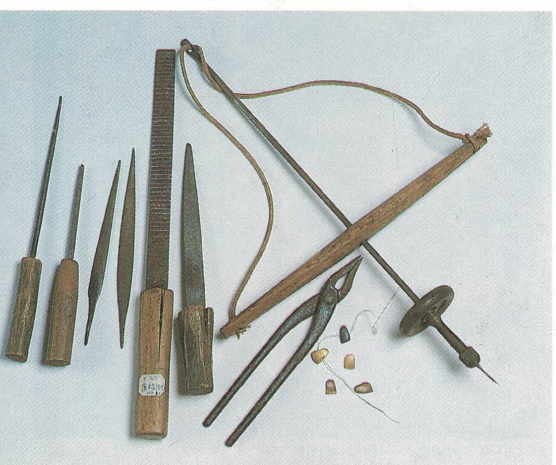
6 歯型彫刻用器具 Tools for carving artificial teeth.
