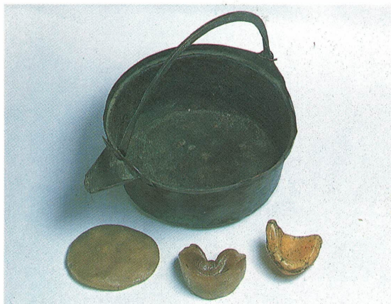
1 蜜蠟軟化用鍋と蠟模型(陰陽型) Pot for softening beeswax and beeswax moulds.
